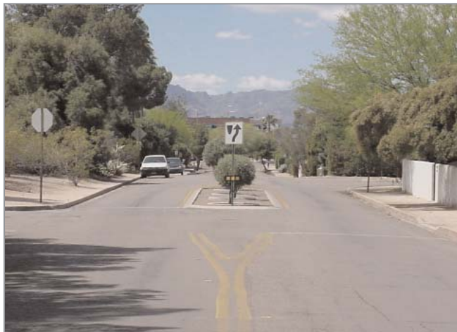
Tree-lined medians and small chicanes reduce drivers' perceived speeds on Elm Street.
