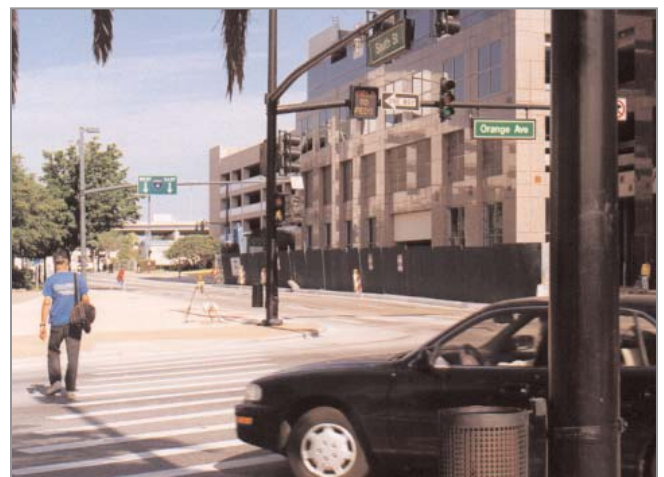
With the 4 second lead time given by the leading pedestrian interval, pedestrians are able to cross part of the intersection before vehicles begin turning.
