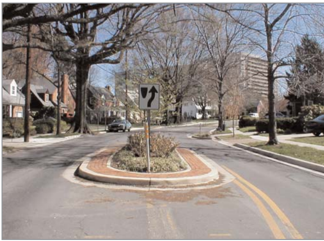
Chicane with median island creating serpentine design.
