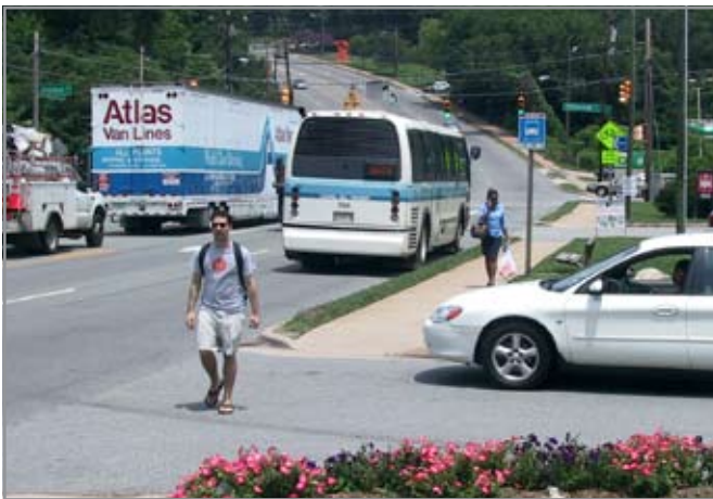
Transit stop placement can impact sight distance at junctions.
