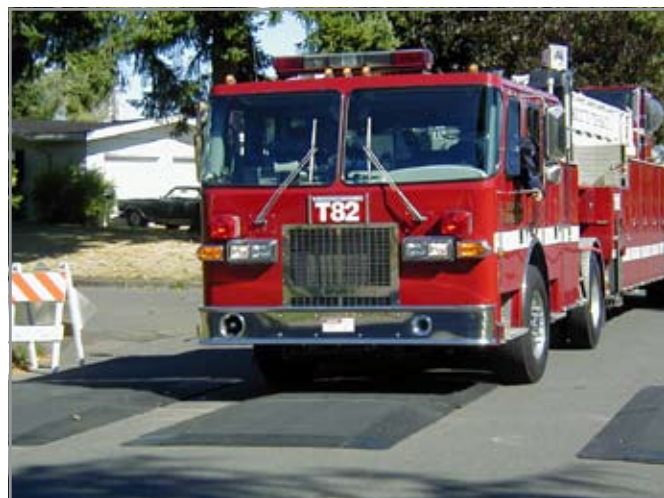
A speed cushion is placed longitudinally in the travel lane. Vehicles with wider axles straddle the cushion.
