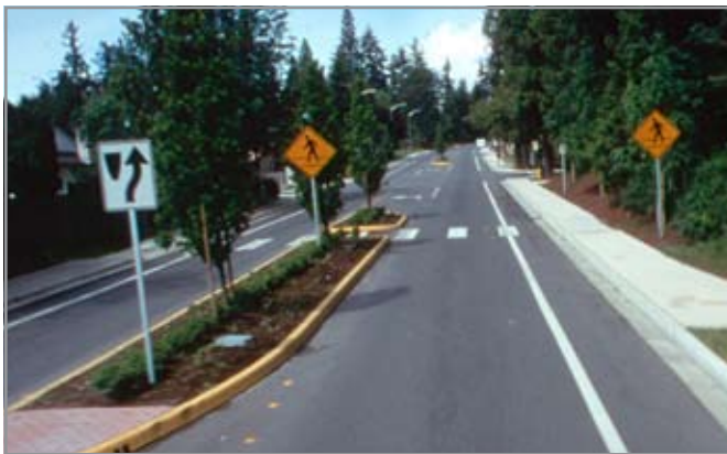
While this median treatment provides a crossing point and a refuge for pedestrians, space is still available for bicyclists.
