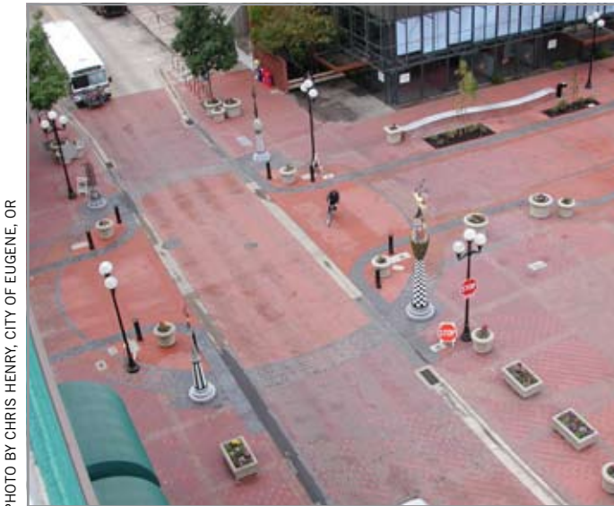
Street furniture was used to visually narrow the roadway through this plaza in Eugene, OR.
