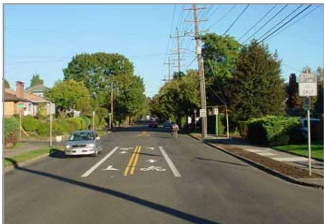
A bicycle-only center-turn lane in Portland, OR, helps bicyclists navigate an offset intersection.
