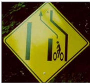
Warning sign alerts bicyclists and motorists to an upcoming lane shift.
