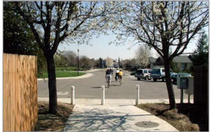
Bollards restrict motor vehicles from a neighborhood connector between cul-de-sac streets.
