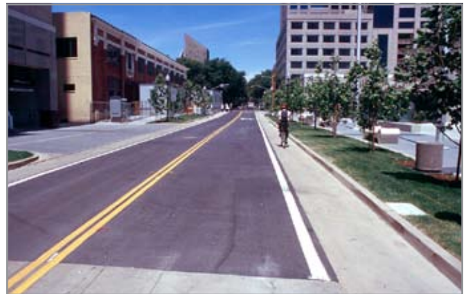
Use of contrasting paving materials highlights this bike lane and visually narrows the roadway space in Sacramento, CA.
