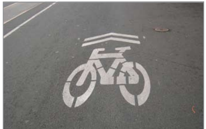
The “bike and chevron,” or SHARROW, is used to indicate both the presence of bicycles and the correct placement of bicycles in the traffic lane.
