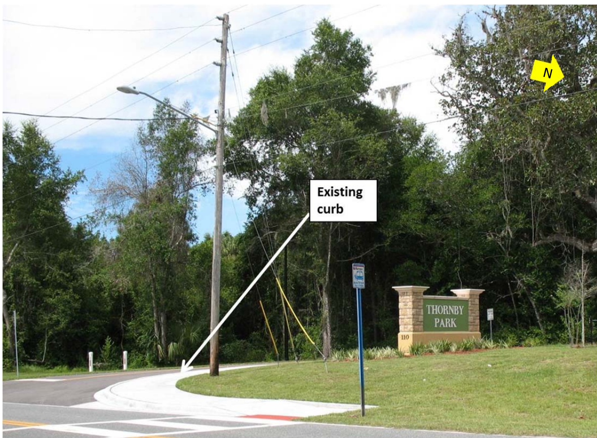
Figure 9: A curb ramp and utility adjustments will be necessary for the trail to cross the driveway of Thornby Park.
