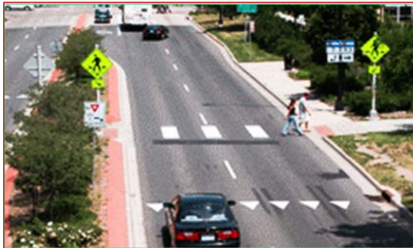
Figure 10: Picture of R1-5a Crosswalk Sign in combination with Yield Lines (source: http://www.bouldercolorado.gov/index.php?option=com_content&view=article&id=963&Itemid=3625 )
