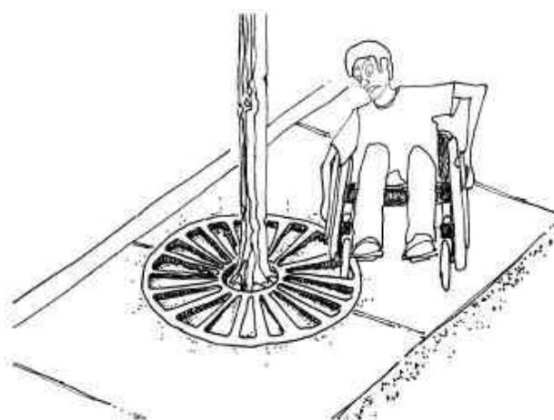
Figure 4-12: Wheelchair casters and cane and crutch tips can easily get caught in wide grates.
