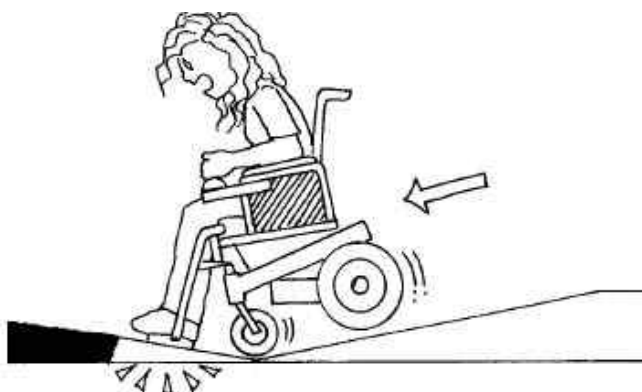
Figure 4-3: Excessive slope differences between gutter and ramp can cause a wheelchair to tip forward.
