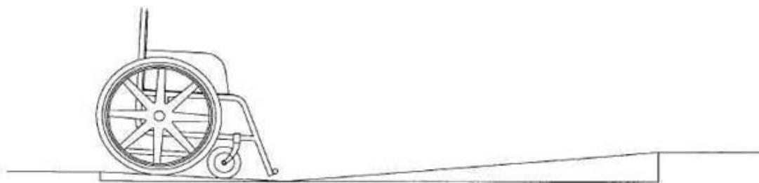
Figure 4-2: The gutter slopes counter to the slope of the curb ramp to promote drainage.
