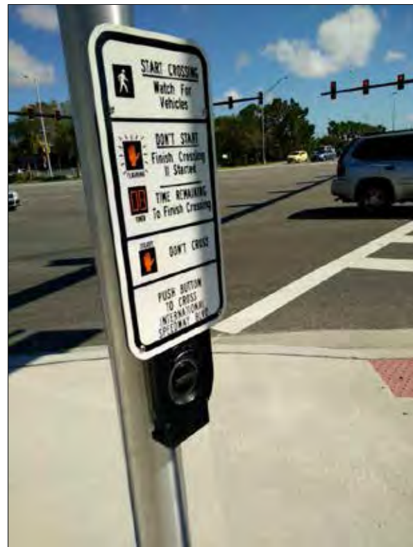
Figure 1 Accessible Pedestrian Signal devices at International Speedway Blvd and Williamson Blvd in Daytona Beach, FL
