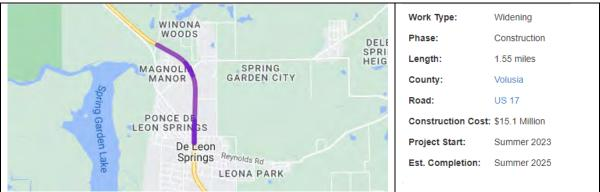
The purpose of this project is to increase capacity and enhance safety along U.S. 17/State Road (S.R.) 15 from south of Spring Street to Lake Winona Road. The project widens U.S. 17 from two lanes to four lanes to enhance mobility in the area. A new roundabout at the intersection of U.S. 17 and Spring Garden Avenue/Spring Garden Ranch Road is also being constructed to improve operations and safety.
