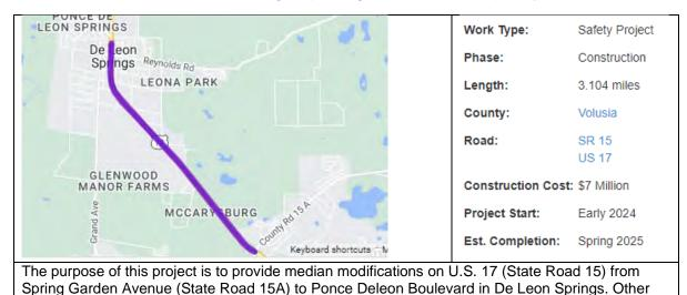
improvements include repaving, drainage modifications, sidewalk and pedestrian curb ramp reconstruction, updated signage and striping, and lighting improvements. There are currently no lane closures.
