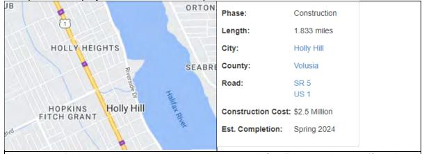
The purpose of this project is to implement improvements on U.S. 1 (Ridgewood Avenue/State Road [S.R.] 5) at the intersections of 6th Street, 8th Street, Walker Street, and Flomich Street in Holly Hill, Volusia County. The existing concrete strain poles supporting the traffic signals at each intersection will be replaced with steel mast arms. Work also includes resurfacing the roadway within each
