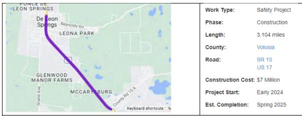
The purpose of this project is to provide median modifications on U.S. 17 (State Road 15) from Spring Garden Avenue (State Road 15A) to Ponce Deleon Boulevard in De Leon Springs. Other improvements include repaving, drainage modifications, sidewalk and pedestrian curb ramp reconstruction, updated signage and striping, and lighting improvements.
