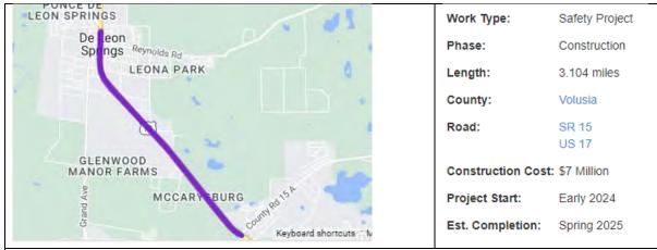
The purpose of this project is to provide median modifications on U.S. 17 (State Road 15) from Spring Garden Avenue (State Road 15A) to Ponce Deleon Boulevard in De Leon Springs. Other improvements include repaying, drainage modifications, sidewalk and pedestrian curb ramp reconstruction, updated signage and striping, and lighting improvements.
