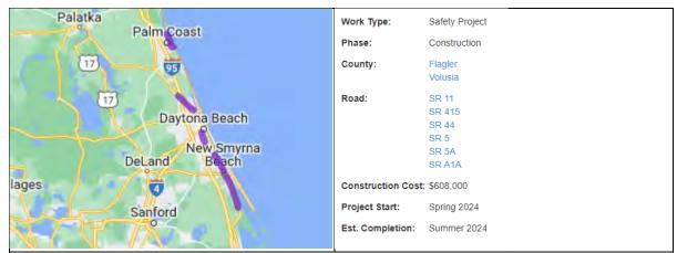
The purpose of this project is to enhance safety along select segments of state roadways in Volusia and Flagler Counties by installing sinusoidal rumble striping and pavement markings along the travel lane lines. The rumble stripes help to alert drivers if the vehicle moves outside the travel lane by creating vibration and noise.
