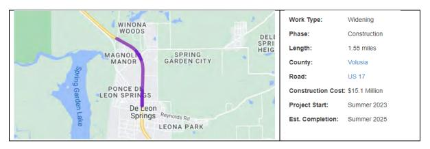
The purpose of this project is to increase capacity and enhance safety along U.S. 17/State Road (S.R.) 15 from south of Spring Street to Lake Winona Road. The project widens U.S. 17 from two lanes to four lanes to enhance mobility in the area. A new roundabout at the intersection of U.S. 17 and Spring Garden Avenue/Spring Garden Ranch Road is also being constructed to improve operations and safety.
