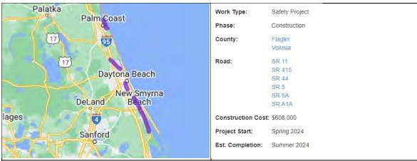
The purpose of this project is to enhance safety along select segments of state roadways in Volusia and Flagler Counties by installing sinusoidal rumble striping and pavement markings along the travel lane lines. The rumble stripes help to alert drivers if the vehicle moves outside the travel lane by creating vibration and noise.
