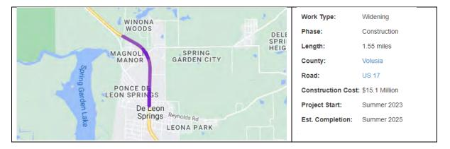
The purpose of this project is to increase capacity and enhance safety along U.S. 17/State Road (S.R.) 15 from south of Spring Street to Lake Winona Road. The project widens U.S. 17 from two lanes to four lanes to enhance mobility in the area. A new roundabout at the intersection of U.S. 17 and Spring Garden Avenue/Spring Garden Ranch Road is also being constructed to improve operations and safety.
