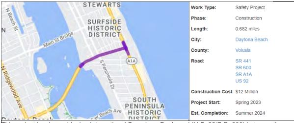
This project involves widening International Speedway Boulevard (U.S. 92/S.R. 600) between the Halifax River Bridge and S.R. A1A to provide two travel lanes, a 6-foot-wide sidewalk headed westbound, and a 10-foot-wide sidewalk headed eastbound. Improvements also include resurfacing
