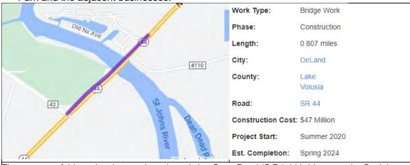
The purpose of this project is to replace the existing State Road (S.R.) 44 bridge over the St. Johns River, also known as the Whitehair Bridge, with a high-level fixed span bridge. During construction, the existing S.R. 44 bridge will remain open for drivers to use while the new bridge is constructed to the south of the existing bridge. After construction, the existing bridge will be removed.
