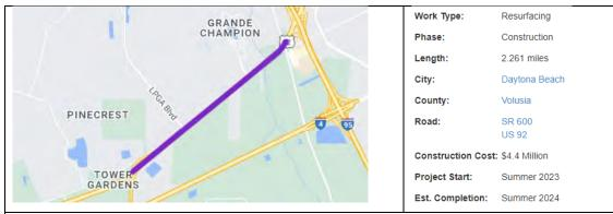
The purpose of the project is to repave this segment of International Speedway Boulevard (U.S. 92/S.R. 600) from north of Educators Road to north of Tomoka Farms Road to rehabilitate the asphalt pavement and extend the life of the existing roadway.
