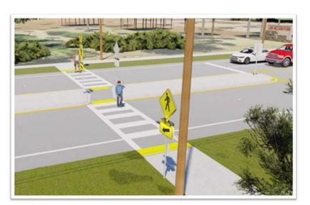
The project also plans to construct raised islands in three short segments (85 to 110 feet long) to encourage slower driving speeds and help enhance safety for pedestrians crossing S.R. A1A. Locations for the raised islands are north of Wren Road, north of Northshore Drive, and north of Byron Ellis Drive.
